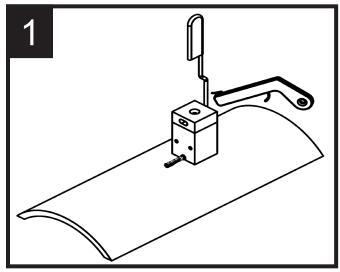
Make your exothermic connection using thermOweld® brand welding products.
