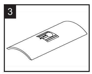
Apply the thermOcap PC to the pipe by pressing firmly on all edges to insure a proper connection.
