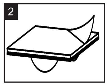
Peal backing from the thermOcap PC using the attached tag.
